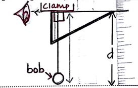
Fix the set square exactly where the [1] string begins. Place a ruler at the other end of the set square as shown. View from the left of the set - up and mark off the measure
